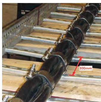
After short circuit test
