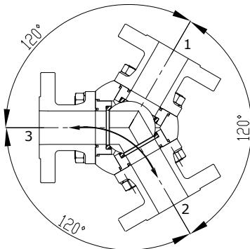
Position-2 (Counterclockwise rotation) flow from 3 to 2
