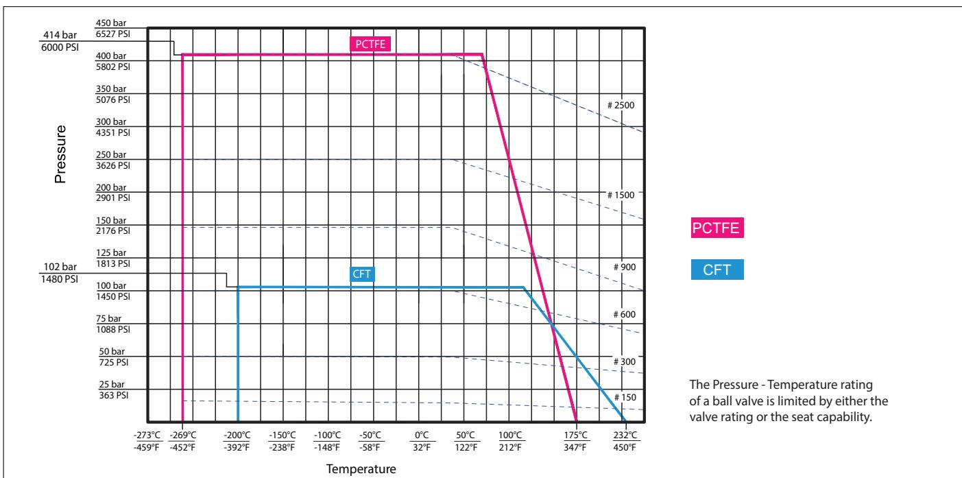
The Pressure - Temperature rating of a ball valve is limited by either the valve rating or the seat capability.
