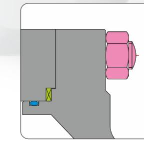
Double sealing on body joints
